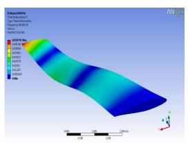
Fig 16: Contour of Mode shape 5
