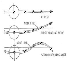
Fig 2 Wing vibration mode shapes
