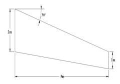
Fig 4.: taper wing dimensions
