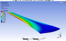
Fig 15: Contour of Mode shape 4
