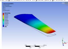
Fig 10: Contour of total deformation on wing Stresses due to fluid pressure
