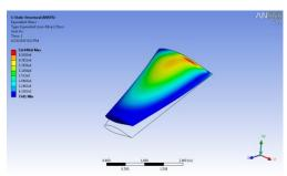
Fig 11: Contour of Von-mises stress
