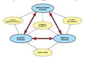
Fig 1: the Collar's aero elasticity Triangle
