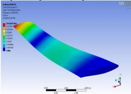
Fig 14: Contour of Mode shape 2
